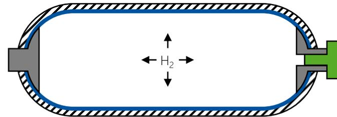
Fig. 3: Hydrogen pressure vessel (Yamashita et al. 2015; Lengersdorf 2017)
