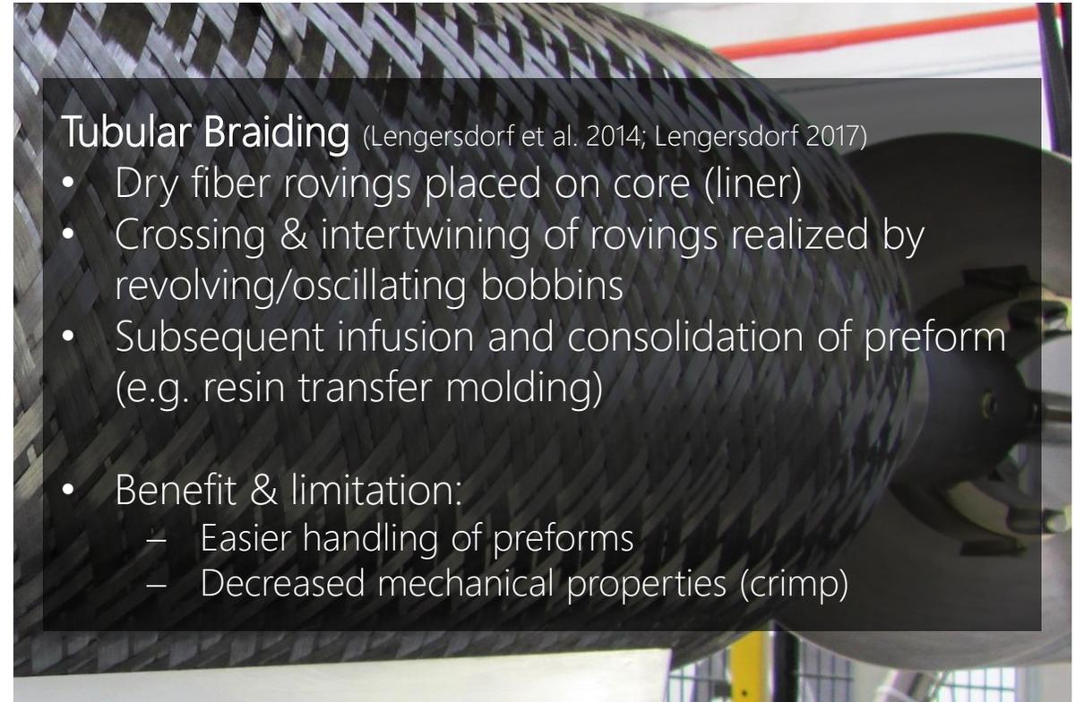
Fig. 5: Tubular Braiding of pressure vessel (Moore 2020)
