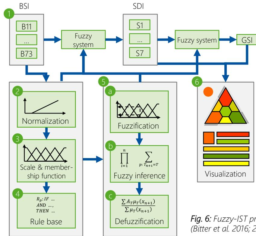
Fig. 6: Fuzzy-IST process (Bitter et al. 2016; 2017)
